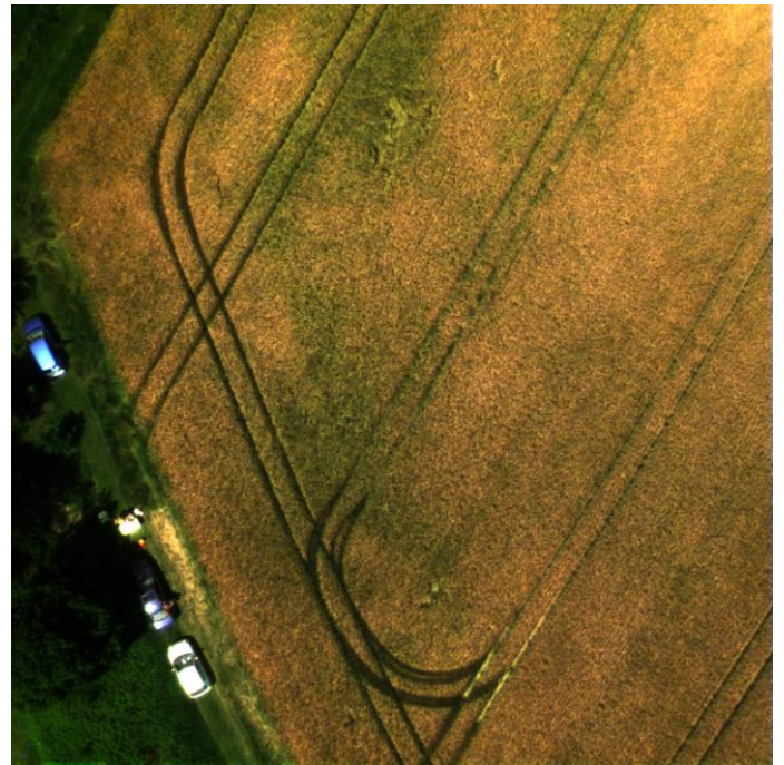
ULTRIS Plus True Color, pansharpened product (factor 4.6, bicubic), 1880x1800 pixel, 100 spectral bands
