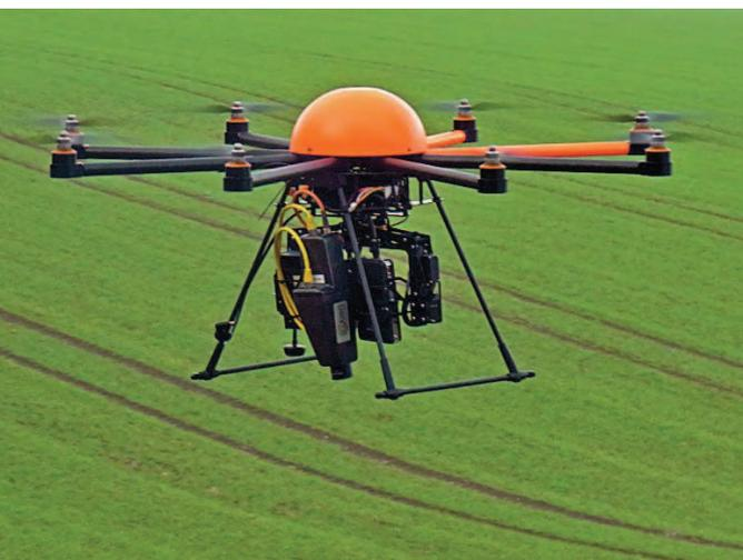
*Left: The UHD 185 records one image per second until the whole area was captured. The octocopter flies in an altitude of 30 – 100 m with a speed of 5 -20 km/h.*
